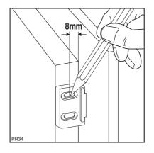
Remove the little plates and make the holes with a diam. of 2 mm. Replace the little plates over the runners and screw in the screws provided (3.5x16 mm).
